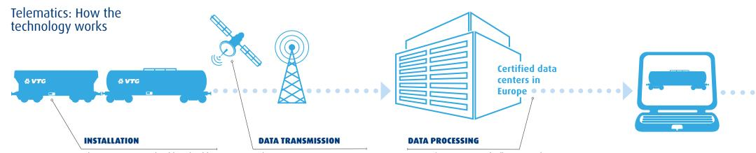
The VTG Connector should preferably be affixed to the I-beam of the wagon. Solar cells combined with a built-in battery guarantee a stable power supply.
