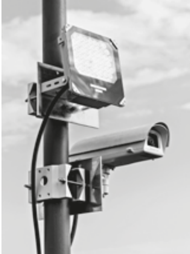
A RailWatch camera identifies the passing wagon
