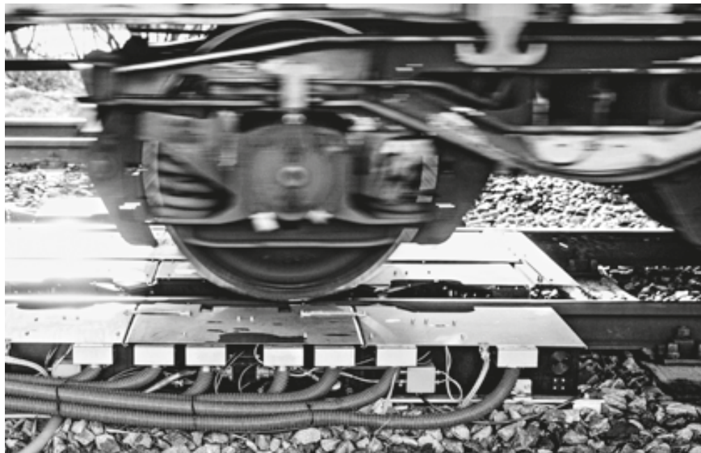
The modules in the measuring station scan the passing train automatically
